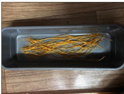
Figure1. Extraction of Bamboo Fibre from The Bamboo Strip
