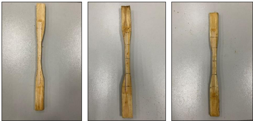
Figure 6. Mode of Failure Tensile Specimen
