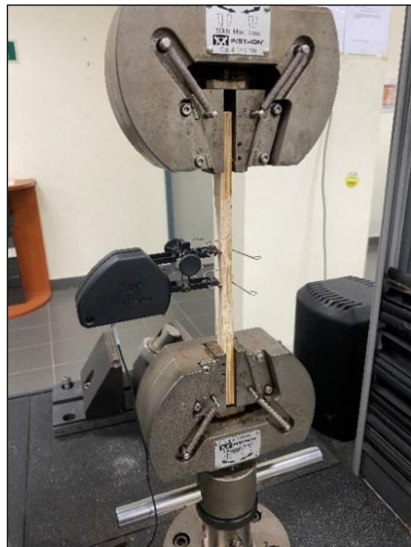
Figure 4. Illustrates The Setup for Conducting The Tensile Strength Test
