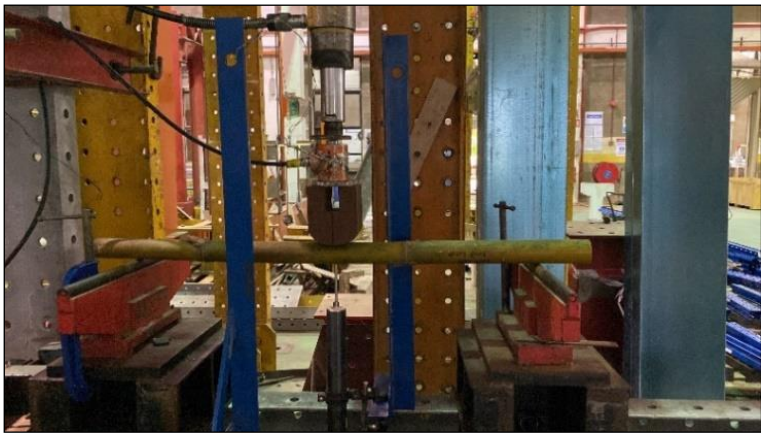
Figure 5. Illustrates The Setup For Conducting The Bending Test
